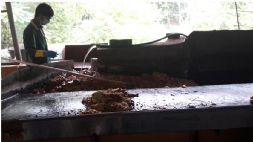
Fig. 18.11 Feeding arrangement in the biogas plant
